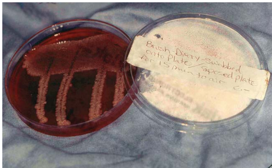
Figure 2. An agar plate was directly swabbed with a used cleaning brush. After being swabbed, the plate was exposed to ambient air for 15 minutes, covered, and then incubated.
